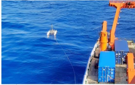
IOW Kat 1200 kHz ADCP & CTD Chain
