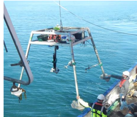
Tidal and plume dynamics: ADCP Lander SedObs mit Pop-Up Bojen in ~30m: Upward 600kHz, 12kHz ADCP, LISST 100X, CTD, downward 1200kHz ADCP
