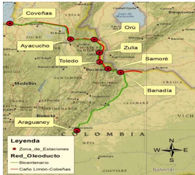
Figure 22. Bicentenario Oil Pipeline Map
