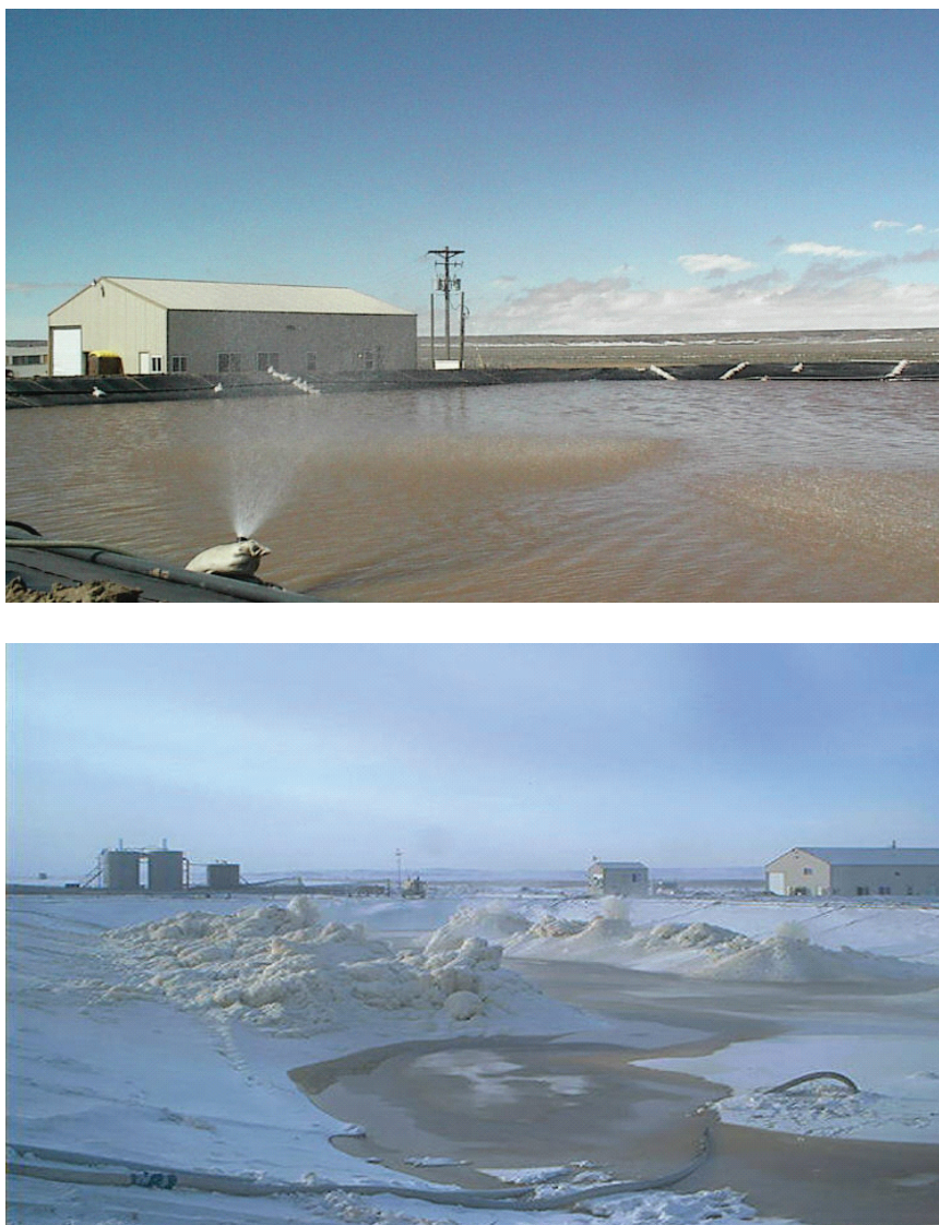
FIGURE 6.2 Seasonal cycle for freezing, thawing, and evaporation of produced water in Wamsutter, Wyoming. Top: Summer evaporation of melted, relatively pure ice. Bottom: Winter freezing of produced water solution to result in relatively pure water in the form of ice crystals. SOURCE: Used with permission from John Boysen, BC Technologies, Ltd.
